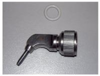
Assemble nozzle into retaining nut
