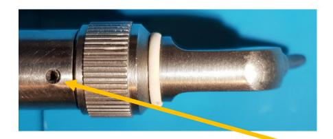
Ensure that the internal part has not rotated. It is held in place with a grub screw that is visible in the small hole next to the nozzle.
